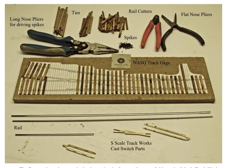
The first step is to glue your ties in place using the free templates, available on the S Scale Track Works web site, as a guide. I used white PVA glue for the template and the ties. I like to pre stain my ties. Some people like to sand the tops of the ties once they are in place so staining after they are sanded makes more sence. Do what works best for you.
